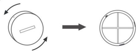
Anticlockwise rotating the battery cover to open
