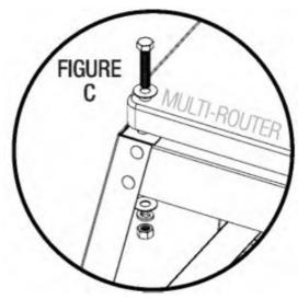
5. Adjust Legs so that they are even and flat on the ground. Tighten the Nuts on all Leg/Stretcher joints.
