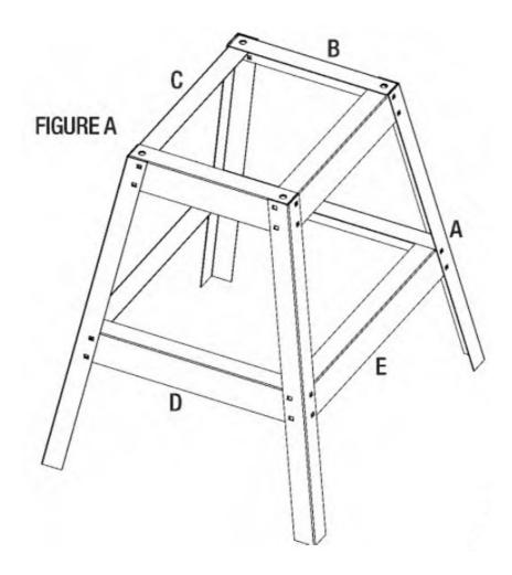
2. From the outside, install  $5/16''-18 \times 3/4''$  Carriage Bolts through all holes. Place a 5/16'' USS Washer and a 5/16''-18 Hex Nut on each Carriage Bolt, finger tight only. Figure B.
