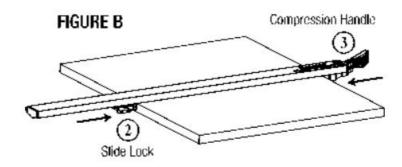
Close the Compression Handle completely. You'll notice there is a "half-way" stop of the Compression Handle. This partially locked position allows you to make fine adjustments to the position of the Clamp-N-Guide before closing the Compression Handle completely.
