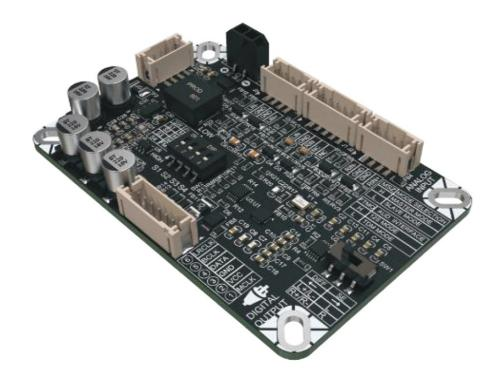
The ASCM-A2D is an audio analog-to-digital module that is designed to enable the sampling two analog channels simultaneously. ASCM-A2D also supports single-ended and differential signals.
