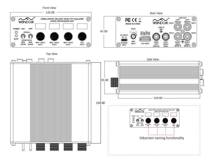
The empty space in the silkscreen on the front panel, as depicted in the picture, can be filled with the functional name of the potentiometer using a marker or sticker for your reference.
