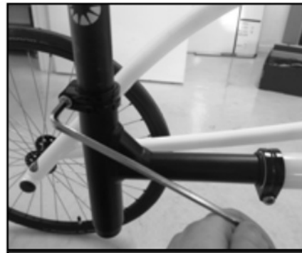
Image 7 Loosen the bolt to height adjust
