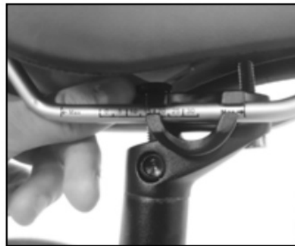
Image 9 Turn the bolt to angle adjust
