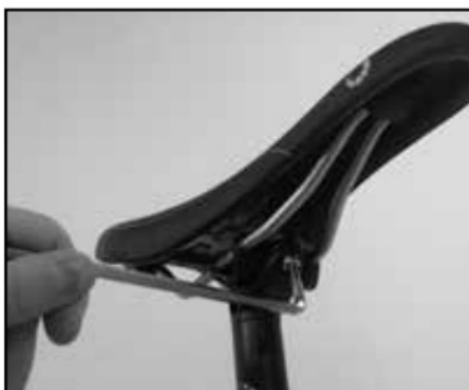
Image 8 Loosen the bolt to angle adjust
