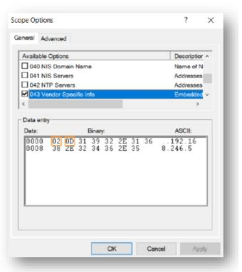
0x02 = Type Cynap Devices (defined by WolfVision) 0x0D = decimal 13 in hex = length of the IP address (4 octets, inclusive dots)
