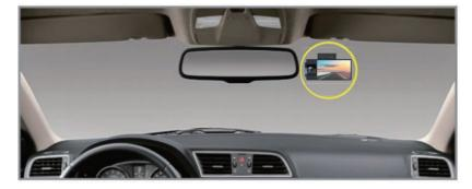
2. Make sure to clean your windshield from the dust particles and attach the electrostatic sticker to the windshield.
