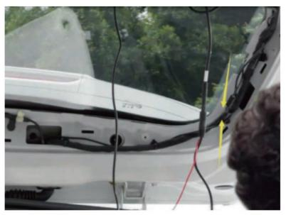
5. Route your rear camera's power cable to the front of the car. If you'd like, use a trim removal tool to pop out the headlining panel directly above your windshield.
