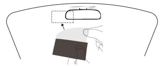
3. Peel off the 3M tape attached to the GPS built-in bracket and attach it on the electrostatic sticker on the windshield.
