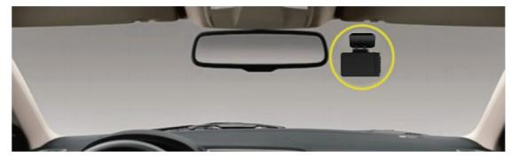
2. Make sure to clean your windshield from the dust particles and attack attach the electrostatic sticker to the windshield.
