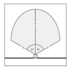
The sensor senses up to 5m and up to 60°, vertically.
