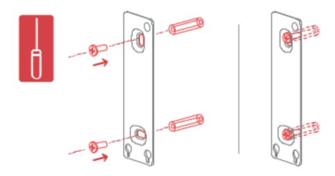
Step 4: Attach Keypad Touch to Mounting Plate
