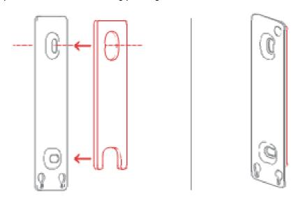
**Step 3: Attach Keypad Touch to Mounting Plate**
