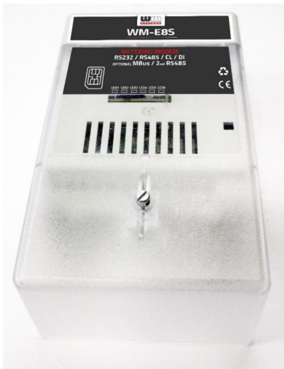
WM-E8S modem, assembled with housing and IP52 protected transparent cover
