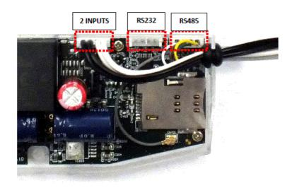
**Order option**: 2 INPUTS – order option – 4-pin connector, connected to the CN502. The cable outfit leads to a 4-wire connector to connect to the external devices. Pinout: black wire is related to input nr. #1, white wire is related to input nr. #2.
