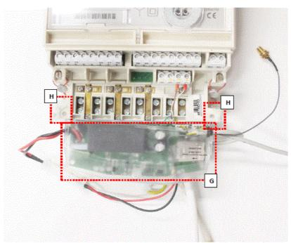
Step #7: Replace the terminal cover on the meter, slide it on, and secure it with the two screws.
