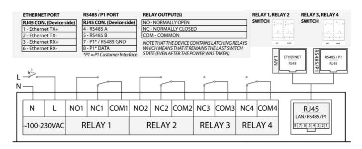
CAUTION! DO NOT CONNECT ~100-240V AC POWER SOURCE to the pigtail AC CONNECTOR (24) OR THE POWER INPUT (12) OF THE DEVICE until you did not finished with the wiring! WHEN OPEN THE ENCLOSURE, ALWAYS ENSURE THAT THE PCB IS NOT CONNECTED TO THE POWER SOURCE and the supercapacitors are exhausted (LED SIGNALS ARE INACTIVE) BEFORE TOUCH THE PCB!
