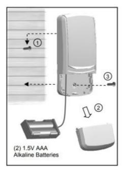
When the battery of Keyless Entry is low, dimmed illumination is observed. To replace batteries, remove the battery cover, replace the batteries with (2) 1.5V AAA alkaline batteries.
