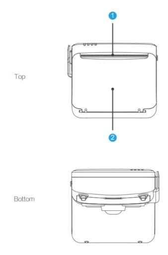
1. 58mm Thermal Printer 2 Contactless Card Reader
