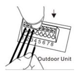
Press down on the button, and insert the wire in the corresponding hole. Release the button to clamp the wire in place.
