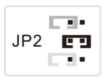
• When removing the jumper cap, it will set the unlock time to 3 seconds.
