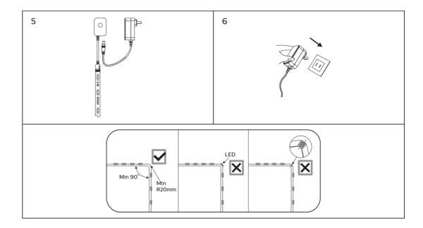
Only use the control box provided in this kit to control this light strip. This lamp will not operate properly when connected to a standard (incandescent) dimmer or dimming control device. The maximum overall length of the light strip should not exceed 33 feet connected to one Wi-Fi controller.
