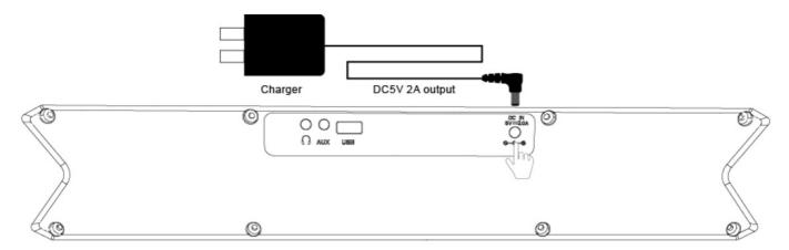
**DC IN:** Charge with DC5V adapter. Only use power adapter we provided to connect MX Gaming 2 ,or i1 may cause burning hazard
