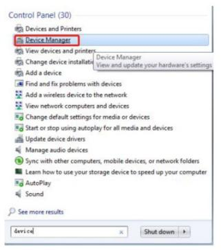
2. After opening the device manager, you will need to open the Ports (COM & LPT) tree. The CH340 should show up as USB-SERIAL CH340 (COM##). Depending on your computer, the COM port may show up as a different number.
