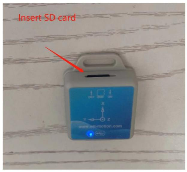
• Step 3. Remove the SD card and insert it into the card reader, than you can check the recoding file as txt.
