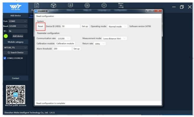
• Click "Reset" if the baud rate or ID is not the default setting (default baud rate: 115200, ID: 0X50), search for the device again.
