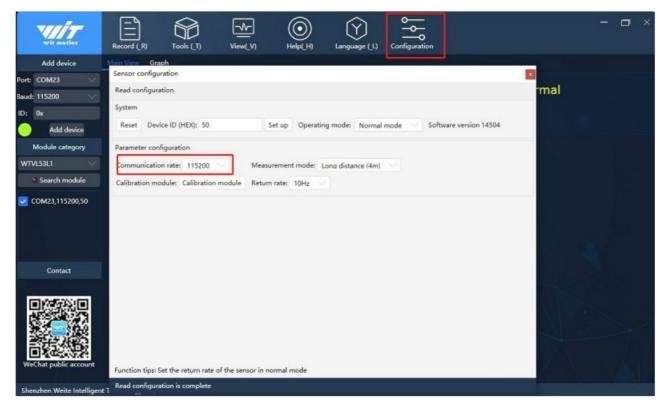
• After the setting is completed, the baud rate of the host computer will be automatically modified.
