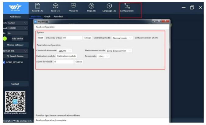
• Click "Alarm threshold" after entering the threshold for Alarm Threshold. The alarm threshold setting range is
