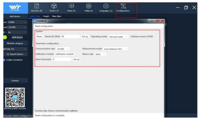
• After entering the device ID, click "Set up". ID can be set in the range 0x00~0x7F.
