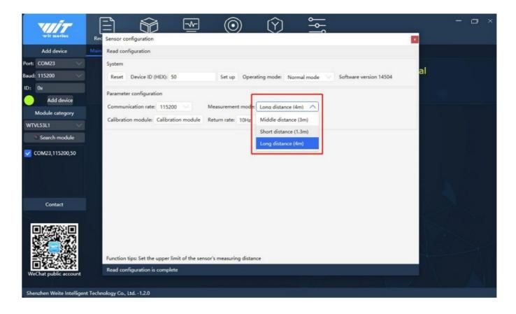
• Click the drop-down box next to the measurement mode to select the corresponding mode.
