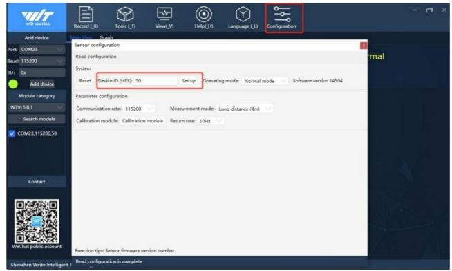
• After setting, other parameters cannot be changed due to the change of the device ID. Click "Search Device" to search for the device again.
