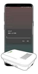
(1) To turn on the wireless motion sensor for the first time, you need to set the Wi-Fi environment throug h the android app.
