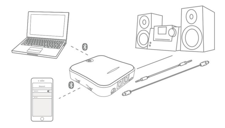
When WISEQ 019 is in RX mode, you can connect WISEQ 019 with a non-Bluetooth audio device like a headphone/ speaker/ audio amplifier via an AUX audio cable or optical audio cable. Then connect WISEQ 019 with Bluet ooth enabled devices like smartphones or laptops etc. via Bluetooth. Therefore, non-Bluetooth audio devices like a headphone/speakers can receive audio signals via Bluetooth.
