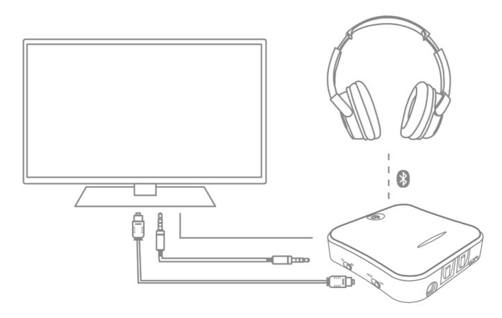
The transmitter mode enables the WISEQ 019 to transmit audio sign al from non-Bluetooth devices like TV or computer to h eadphones or speakers. When WISEQ 019is in TX mode, you can connect WISEQ 019 with a non-Bluetooth audio device like a TV/computer via an AUX audio cable or optical audio cable. Then connect the WISEQ 019 with Bluetooth headset/speakers etc. via Bluetooth.
