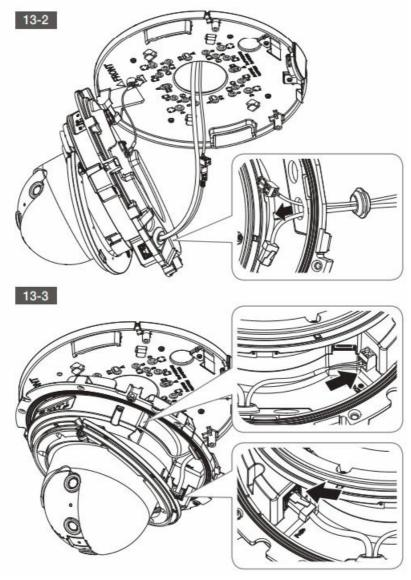
• Installing network cable (PoE)
