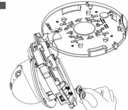
• Installing network/power cables
