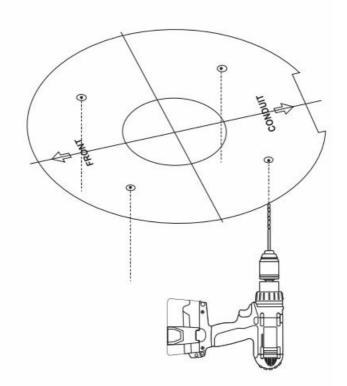
• Directly installing on wall/ceiling
