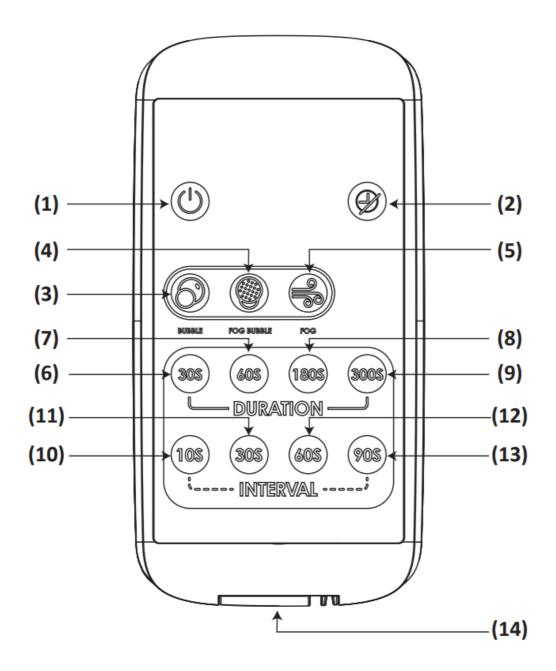
**Timer Settings**: e.g., push the button "30S" of DURATION section and the button "10S" of INTERVAL section, this machine will run 30 seconds in current working mode, then pause 10 seconds, repeat this cycle. Push the button "Timer Off" to cancel the timer settings.
