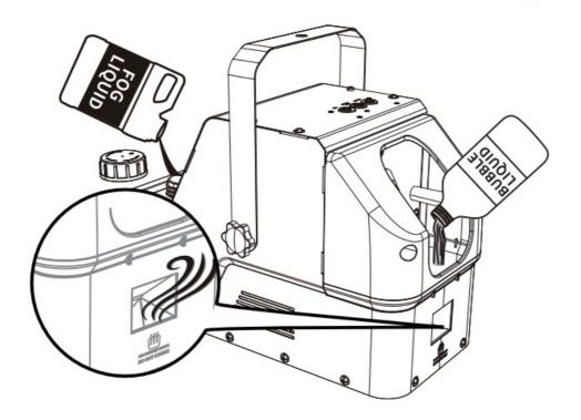
3. Plug the (O) Power Cord into a standard A/C grounded wall outlet and turn on the (M) Power Switch. The (D) LED Status Indicator will turn red approximately 3 to 5 minutes indicating that the machine is heating. When fully heated, the LED status indicator will light off.
