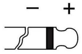
Input Signal: 4-20 volts @ less than 10 mA Output Signal: 12 volts @ 100mA
