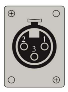
These pin assignments are consistent with the standards adopted by the Audio Engineering Society. Connect the appropriate outputs of your preamp to these inputs, using our WWK-BB8 / CUSTOM-WWK-BB8 balanced audio interconnect kits. If using off the shelf interconnects or making your own cables, only use shielded 3 conductor audio cable.
