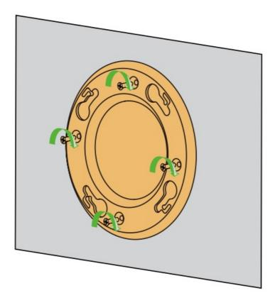
5. Put the device to the mounting bracket, rotate as shown direction to complete the installation.
