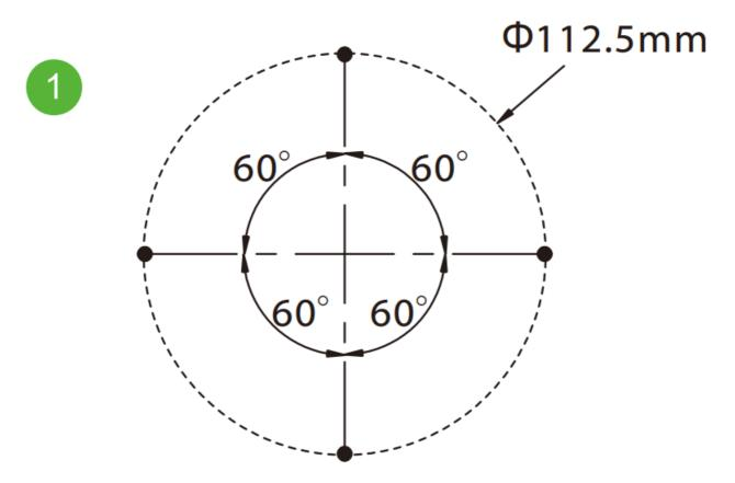
2. Use 6mm drill and drill the hole depth 35-40mm.
