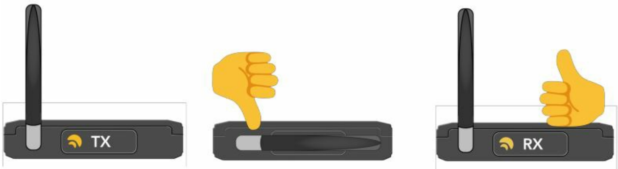
Fig.2: There are limitations to how wireless waves propagate through air. Physical barriers like glass, concrete and walls will limit the transmission range. Always try to have clear line-of-sight between transmitters and receivers.
