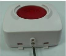
2. Insert the Micro USB programming cable into the M-823 J1.
