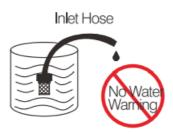
Make sure inlet hose is in the bucket, start the machine in "COOL" mode to avoid machine in dry running and get in dry buming protection. "STEAM" MODE must be used with clean water.
