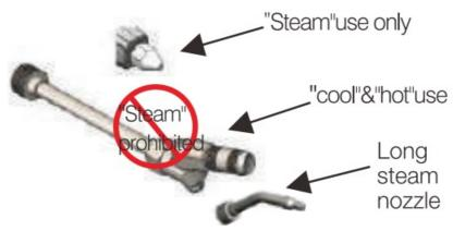
6. Do not touch directly by hand as the internal heater and steam nozzle temperature is very high after using steam and hot water function.
