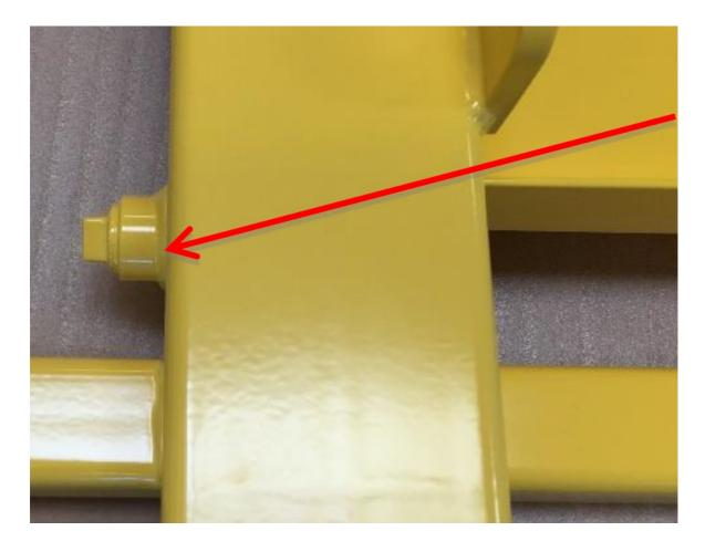
• Remove the two drain plugs (one drain plug on each side). Empty the tank for oil.
