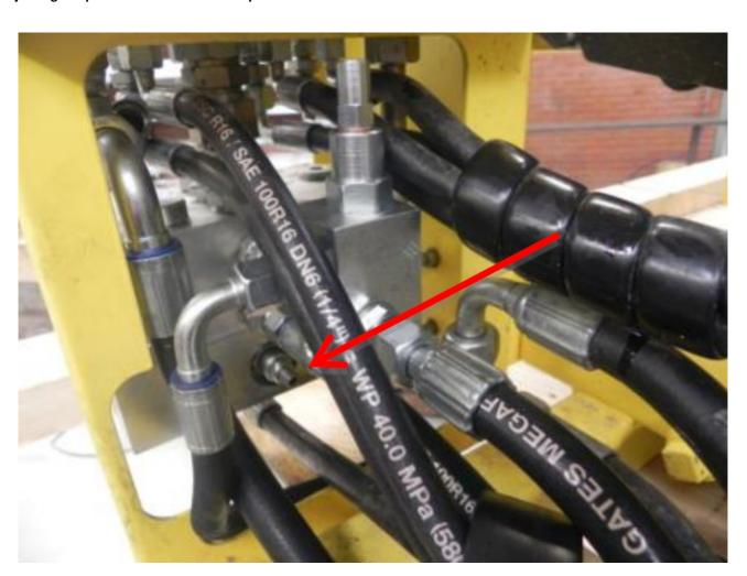
• To adjust the pressure, unscrew the Allen screw. Decrease the pressure by screwing the Allen screw anticlockwise. Increase the pressure by screwing the Allen screw clockwise.
