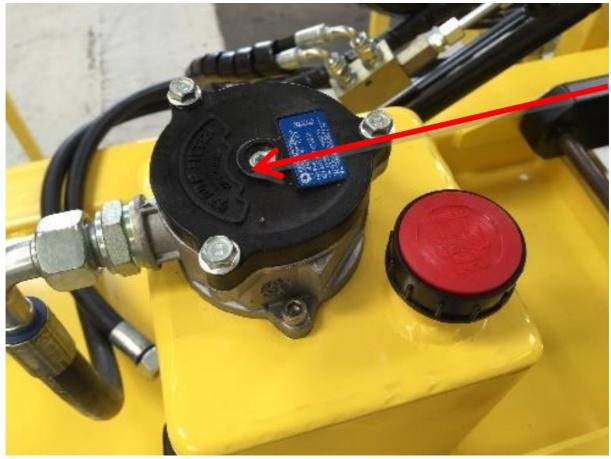
• After 50-100 hours in use the return filter must be changed. Remove the lit of the filter housing. Remove the return filter and insert a new one.
