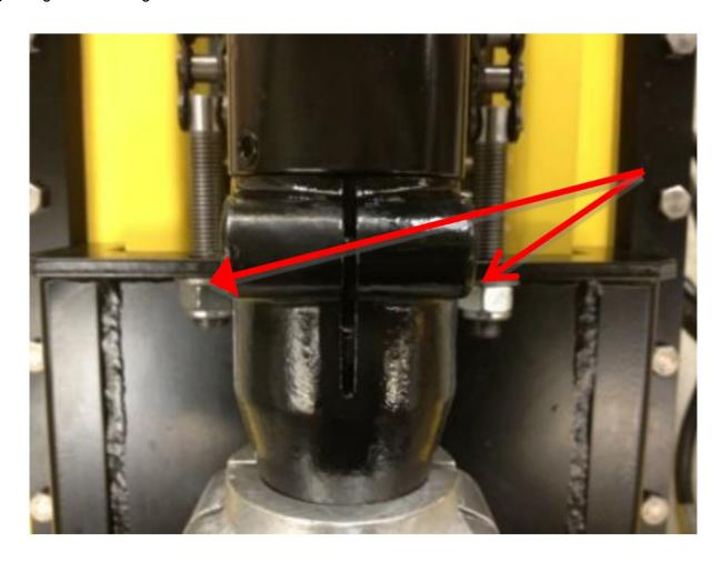
• Tighten the chains by tightening the nuts.
