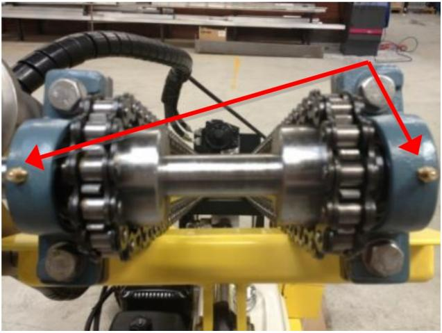
• It is important to lubricate the chain with oil. Lubricate the grease nipples.
