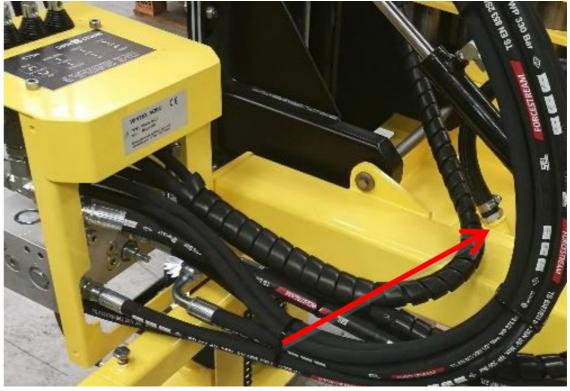
• Remember to check the suction strainer and change it if necessary.
