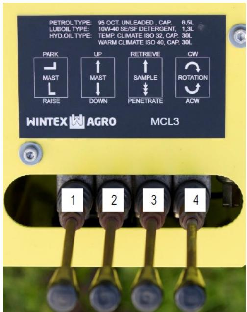
All sampling operations are hydraulically operated from the control panel. There are four separate functions:
