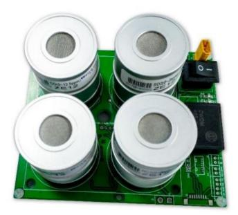
ZEHS04 is a diffusion type multi-in-one module, mounted with atmospheric monitoring module ZE12A, to detect CO, SO2, NO2, and O3. It is also compatible to connect with dust sensor module, temperature and humidity sensor module externally. With TTL or RS485 output, it is convenient to use and debug, which greatly shortens the user's design and development cycle, and meets customers' needs for different gas detection occasions.
