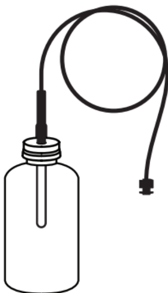
Figure 1: Using a bottle of glycerin as buffer with TEMP-L-S sensor. Sensor sold separately.
