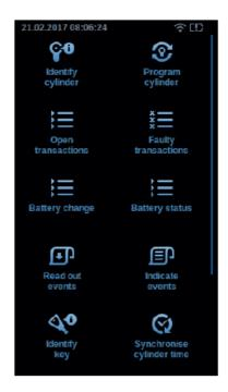
To switch on, please push the on/off switch (9). The ring around the key insertion slot lights up blue and a short beep is heard. Then the Winkhaus logo and a progress bar appear. After that the start window is shown in the display (fig. 3).
