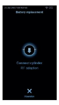
This function is performed after battery replacement took place in one of the components. In the process the time is reset and the counter "Transactions after battery replacement" in the component is set to zero. During the next communication between the BXP and the administration software this information in the software is updated.
