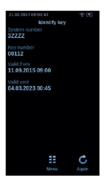
As is the case with the components, you can also have the ID media (keys, cards, key fobs) identfied and assigned. To this effect, please enter the key to be identified into the BXP key slot. Cards and key fobs are placed on the device.
