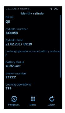
If the locking system or the locking number should no longer be readable, the cylinder, the readers or the fittings (components) can be identified. For instance, connect the BXP to the cylinder and select "Identifying component". The action is automatically started. All relevant data is indicated (see table). Scroll down for further information. **Indicated information**
