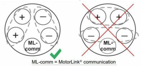
Furthermore, when using a 5-core cable, the distance between "-" and "Com" must be the same as the distance between "+" and "Com". Meaning if L2 e.g. is being used as "Com" L1 and L3 must be used for "+" and "-". When
