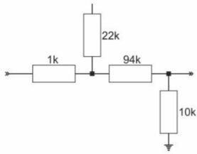
For WCC 310 0410 with only 4 motorlines input X5-X8 have no function. With the default values are input: "Active" if the contact resistance is smaller than  $2k\Omega$  "Inactive" if the contact resistance is bigger than  $3k\Omega$ . Input has pull up current of approx. 0.8mA. (min 0.7mA, max 1mA) Example: comfort keypad connected to input X3
