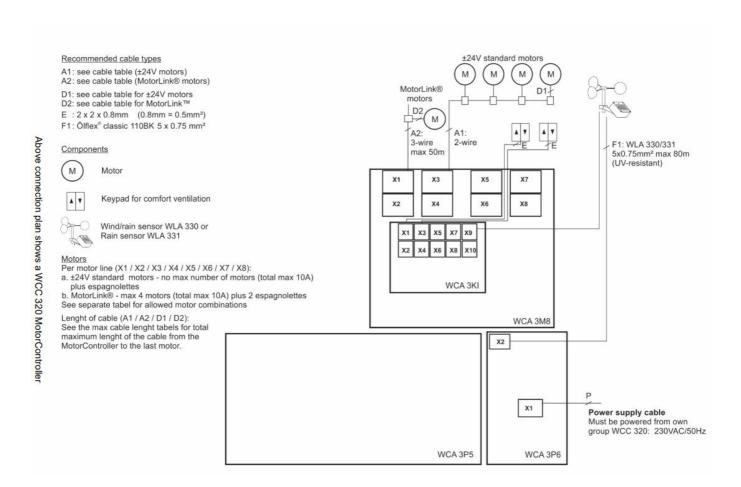
Each motor controller includes a main power supply unit (SMPS), an auxiliary power supply (AUX), a motor line card and an input card. The size of the power supply unit determines the number and/or types of actuators, which can be connected to the MotorController. See table with an overview of the max number of allowed actuators per motor line/motor controller (chapter 3.2).
