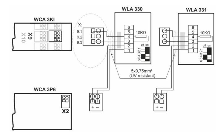
DIP switch 1-3 on WLA 330 must be set for wind speed tolerances. Please refer to the installation instructions for WLA 330 for DIP switch settings. If no wind/rain or rain sensor is connected to S3X9, a  $10k\Omega$  resistor must be connected between S3X9.1 and S3X9.3.
