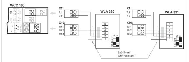
DIP switches 1-3 on WLA 330 must be set in relation to windspeed tolerances. See the guideline for WLA 330 for DIP switch settings.
