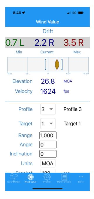
The Wind Drift page displays the current real-time wind drift based on the wind meter readings. The values displayed are the current calculated drift as well as the maximum and minimum values during the previous user-
