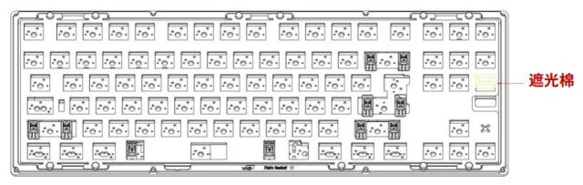
5. Install switches, inter structure, has been built. Put the 2mm portion and 2mm hot swap portion into the bottom case, and connect the PCB with TYPE C.
