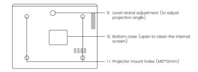
**Note:** For Ceiling mount, please slowly remove the 4 black rubbers, then you can find the holes for ceiling mount. The screw size is M5\*12mm.
