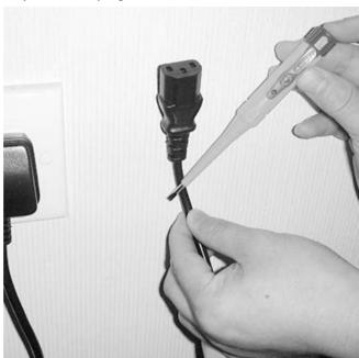
Note: To increase the sensitivity, touch the 'METAL PLATE' while testing.
