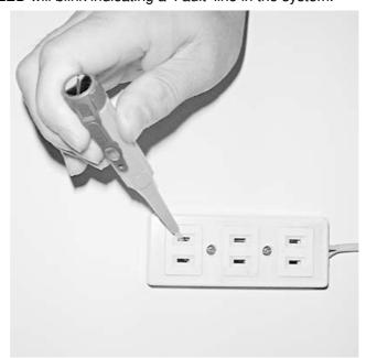
**Note:** When in direct 'Contact Method' mode, it is not recommended to touch the 'Metal Plate' of the tester. (Of course, it is absolutely safe even when touching it.)
