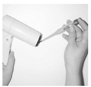
Move the Tester close to hair dryer with the power OFF. 'LED' blinks when the plug is inserted improperly, OR 'LIVE/HOT' wire is connected 'WRONGLY1 to the socket.
