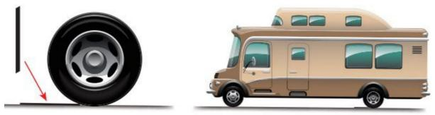
2. Clamp the thin lip of the large wedge between the tyre and rubber mat. This ensures a secure positioning and prevents slipping during the process.
