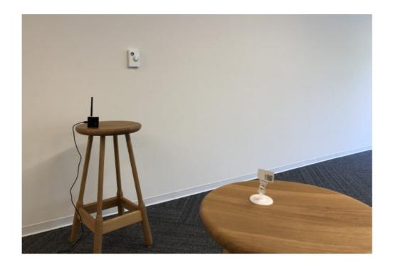
Once the tag is energized it will start transmitting Bluetooth® packets. The gateway will blink red each time it receives a packet.
