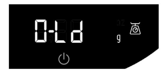
If the scale is overloaded, remove weight from the scale (maximum weight is 2000g).
