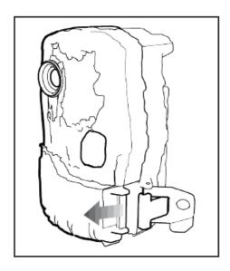
2. Drop the battery tray by sliding the orange EJECT latch to the right.
