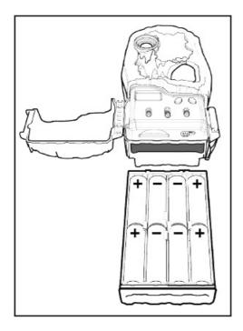
NOTE: Do not mix old and new batteries. Do not mix alkaline, standard (carbon-zinc) or rechargeable (ni-cad, ni-mh, etc) batteries.
