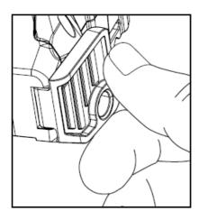
2. With the camera facing open, open the battery compartment cover by sliding the latch to the left.
