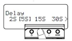
2. Press "ENTER" then use the +/- buttons to choose be-tween 2 seconds, 5 seconds, 15 seconds, 30 seconds, 1 minute or 5 minutes.
