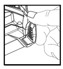
2. Locate the battery compartment and press the "OPEN" tab to the left to open.
