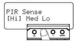
Hi: Detects smallest movements Med: Detects common movements Lo: Detects only large movements
