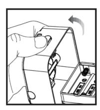
2. Insert the batteries in the appropriate location corresponding to the +/-shown inside the door and above each battery slot.
