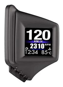
Thanks for purchasing our car smart digital meter. This product connects car OBD2 interface by OBD cable, and display the driving dates, e.g. vehicle speed, engine RPM, water temperature, fuel consumption, voltage etc. It can keep the driver's eyes always on road to avoid the dangerous of lowering down head to read the dashboard. This product won't change any car ECU dates.
