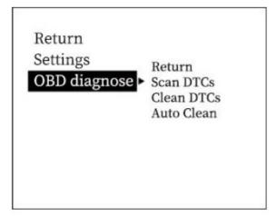
Long press the 'OK'key for 2 seconds to enter the setting item, short press the '>'key to increase the menu option, short press the ok key again to enter the parameter value, short press the '>'or '<'key to adjust the parameter value, short press the 'OK'key to confirm and return Menu, long press the 'OK'key for 2 seconds to save and exit.
