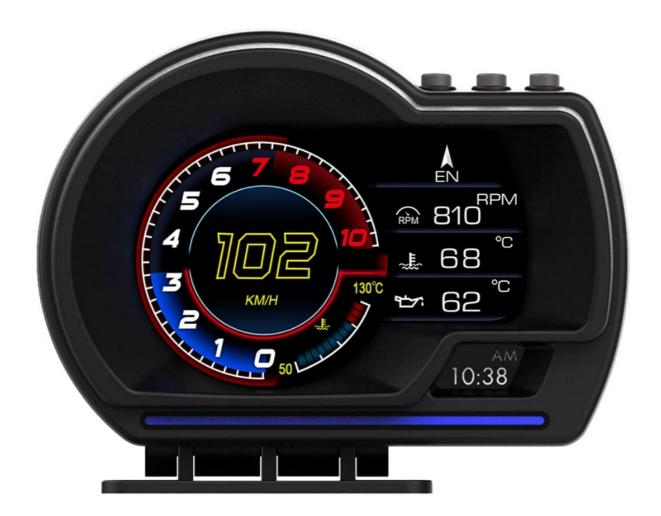
Thank you for purchasing our product this product reads the driving data of the car through the OBD2 interface of the car ECU line computer, such as vehicle speed,RPM, fuel consumption, water temperature and voltage, etc. To keep the driver eyes always on road to avoid the dangerous of lowering down head to read the dashboard. This product does not rewrite any data in the ECU.
