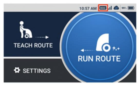
• Please check your mobile phone cellular connection in advance. Robot Operations Center (ROC) will not be connected to LTE in an area where there is no signal.
